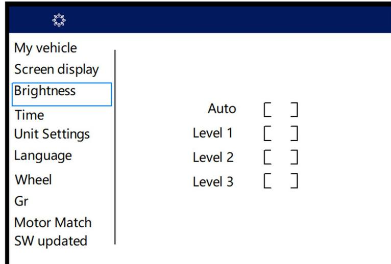
**Brightness:** Press SEL DOWN to enter into “Brightness” setting interface. Then, press SAVE to start selecting the brightness modes by pressing SEL UP or SEL DOWN, and finally, press SAVE to save the setting. There are 4 brightness modes to select. Auto Mode will automatically adjust the brightness accord to the environment luminance. Level 1 is with the highest brightness. Level 1 is with the medium brightness. Level 3 is with the low brightness. Auto Mode is the default setting.
