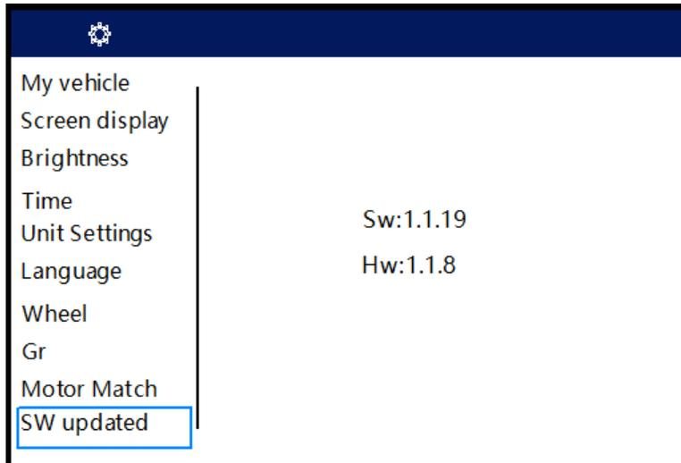
**SW updated:** Press SEL DOWN to enter into “SW updated” setting interface. Press SAVE to select the version number by press SEL UP or SEL DOWN, then, press SAVE to see the information of the Dash’s software.
