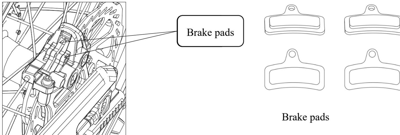
Replace the brake pads when the free clearance of the brake lever exceeds the specified range (15–30mm), Or the total thickness of less than 3mm brake pads, please replace the brake pads.
