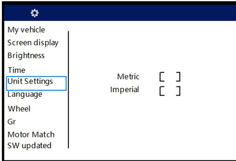
**Unit Settings:** Press SEL DOWN to enter into “Unit Setting” setting interface. Then, press SAVE to start selecting Metric or Imperial unit display by pressing SEL UP or SEL DOWN, and finally, press SAVE to save the setting.
