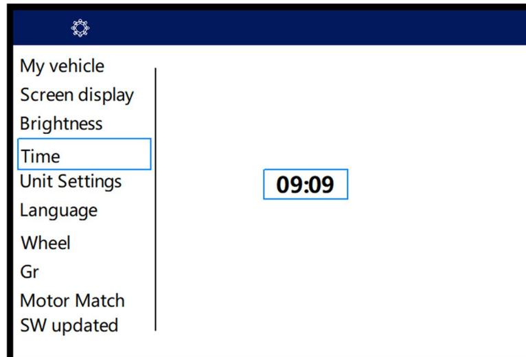
**Time:** Press SEL DOWN to enter into “Time” setting interface. Then, press SAVE to start setting the time by pressing SEL UP or SEL DOWN, and finally, press SAVE to save the setting.
