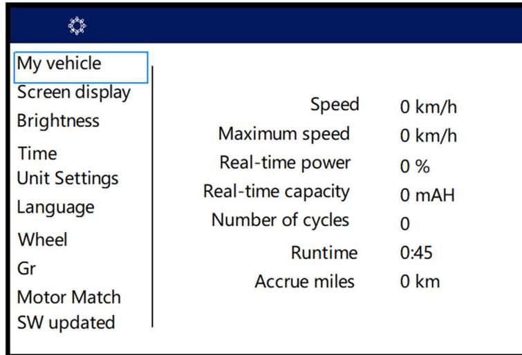
**My Vehicle:** Press SAVE to enter into the set interface, then, the riding data will show on the display (Such as the information about the speed, battery, runtime, range, and so on).
