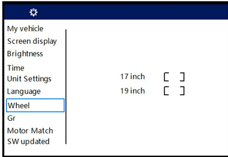
**Wheel:** Press SEL DOWN to enter into “Wheel” setting interface. Then, press SAVE to start selecting wheel diameter by pressing SEL UP or SEL DOWN, and finally, press SAVE to save the setting. The incorrect diameter setting will cause the incorrect speed indication. The default wheel diameter setting is 17inch.
