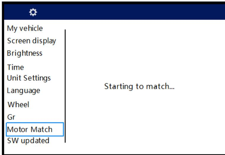
**Motor Match:** Press SEL DOWN to enter into “Motor Match” setting interface. When the motorcycle status is “WAIT”, and the side kick stand is folded up, press SAVE to start the motor match within one minute after the bike is powered on. Then, the motorcycle will have a small move, and after that, it will show the match is successful or failed.
