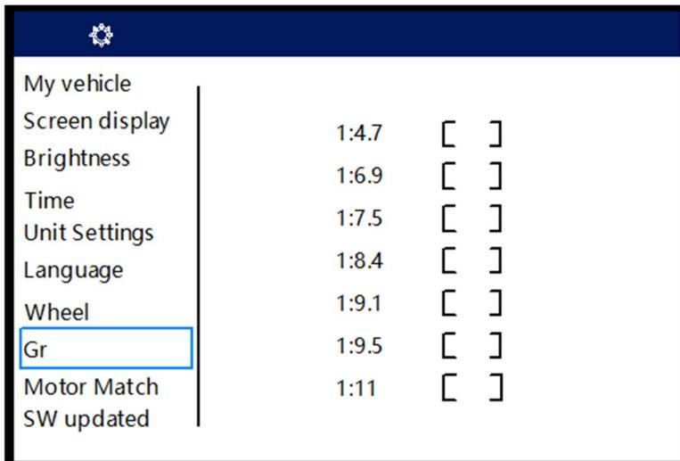
**Gr:** Press SEL DOWN to enter into “Gr” setting interface. Then, press SAVE to start selecting gear ratio by pressing SEL UP or SEL DOWN, and finally, press SAVE to save the setting.
